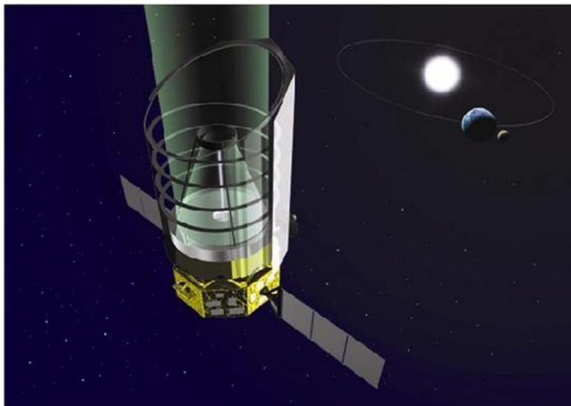
**Figure 2-5** The SPICA Space Telescope is a proposed joint Japanese-European project to develop an advanced far-IR space telescope. It will build on the experience gained from Herschel, but will include significant advances in detector and cryogenic technologies to allow it to be more than an order of magnitude more sensitive than Herschel - anything that Herschel could detect, SPICA will be able to obtain a spectrum of it. (Source JAXA)
