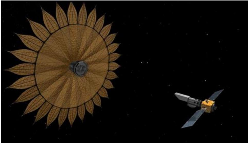
**Figure 2-7 One possible HabEx concept: a star shade is flying in front of the telescope hiding the central on-axis star, while allowing the light of off-axis planets to leak to the telescope. A  $10^{10}$  contrast is achievable with such a design. (Source NASA)**
